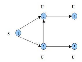
Status of each edge:  $x_j = 0$  if the edge is available, 1 elsewhere. Status of each node:  $x_i = 0$  if the node is connected to at least a source trough at least a path made up of available edges, 1 elsewhere.
