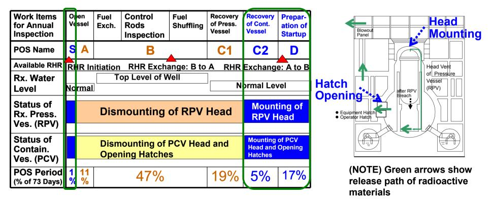
(NOTE) Red triangles show the timings of switching operation for residual heat removal system which is possible to be induced LOCA by human error.
